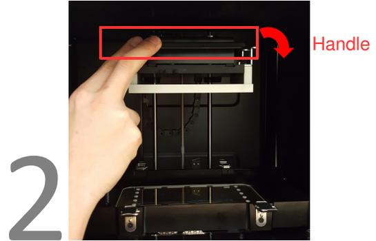
※ Remove the Picker: Lift the handle→Carry both end of picker→Remove the Picker
