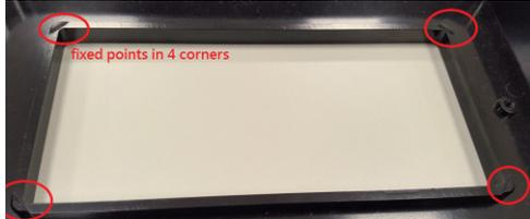
(2) Ensure no residuals inside the tank and the glass is well setup before printing.
