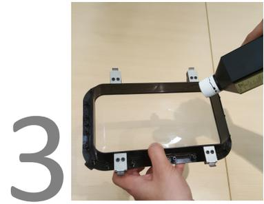
※ Remember to lock four corners of resin tank after install it.
