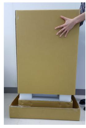
**WARNING** Printer net weighs 37.5kg. Please be careful, and use proper lifting techniques to avoid injury.
